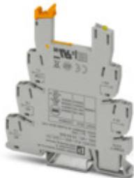
6.2 mm PLC basic terminal block with screw connection, without relay or solid-state relay, for mounting on DIN rail NS 35/7,5, 1 changeover contact, input voltage 12 V DC
