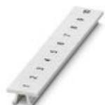
Zack marker strip, Strip, white, labeled, can be labeled with: CMS-P1-PLOTTER, printed horizontally: consecutive numbers 1 ... 10, 11 ... 20, etc. up to 491 ... 500, mounting type: snap into tall marker groove, for terminal block width: 6.2 mm, lettering field size: 6.15 x 10.5 mm, Number of individual labels: 10
