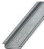
DIN rail, unperforated, Standard profile, width: 35 mm, height: 7.5 mm, acc. to EN 60715, material: Steel, galvanized, length: 2000 mm, color: silver
